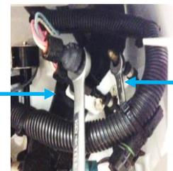
Failure to hold the schrader fitting may cause the feeder line to twist the schrader port, requiring a change of the complete fitting. Perform the same method of retaining the schrader fitting during the install. It is recommended that after you reinstall the fitting that you leak check the connection.
