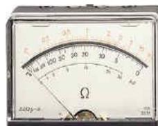
5. Meg at 500 VDC (Note: A megger setting that is higher than 500 VDC may damage the generator windings). A high megger reading (min of 10 megaohms) would indicate a good insulation system.
