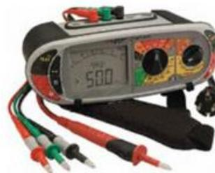
If it is necessary to check the winding insulation resistances between the ground and each lead of the generator to ensure the insulation system of the generator is in good shape. A megger (or meg) test can catch an electrical short to ground where a standard ohm meter would not.
