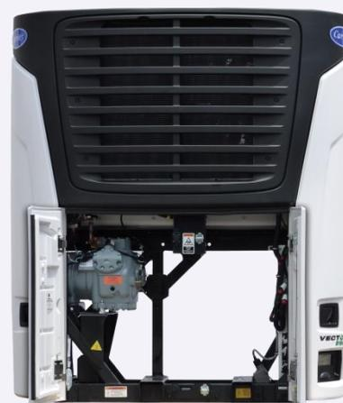
The Vector 5100 (above) is similar to Carrier Transicold's successful Vector 6500 single-temp hybrid unit, minus the diesel engine and associated components.
