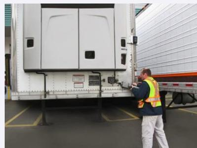
Like an electric refrigerator, a Vector 5100 unit only needs to be plugged into an electric power supply to deliver heating or cooling capacity for perishable or frozen loads.
