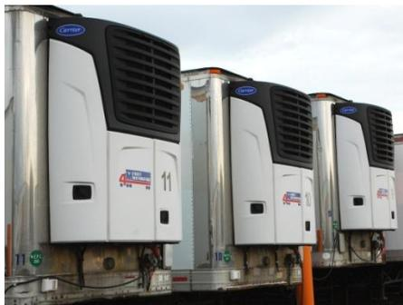
**All-electric Vector 5100 units drive diesel exhaust emissions down to zero because they do not use an engine.**
